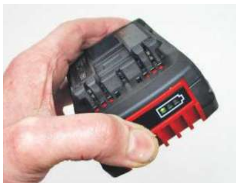
▲ Batteries have a button-operated charge indicator
